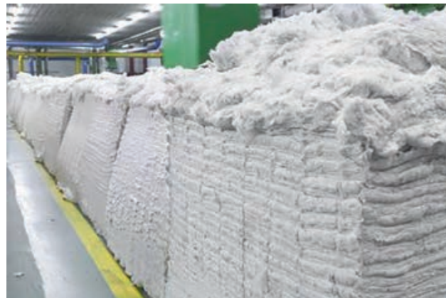
Figure 6 Bale mixing – laydown
