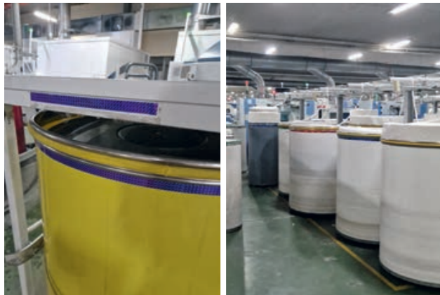
Figure 8 Good identification and mixing of cans from different cards (different color ribbons)
