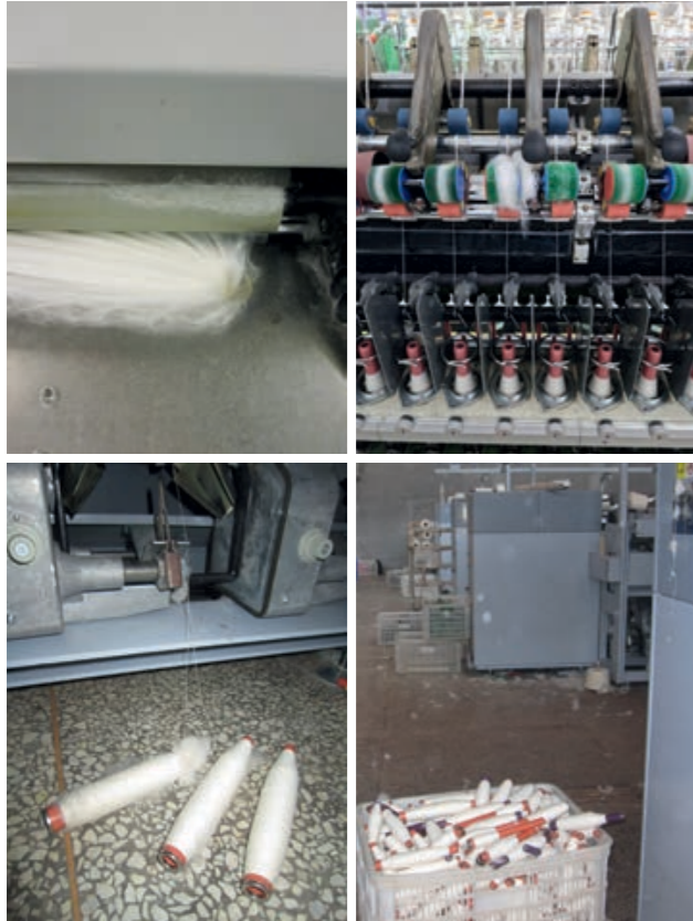
Figure 18 Avoid fiber and dirt accumulation as reason for yarn irregularities
