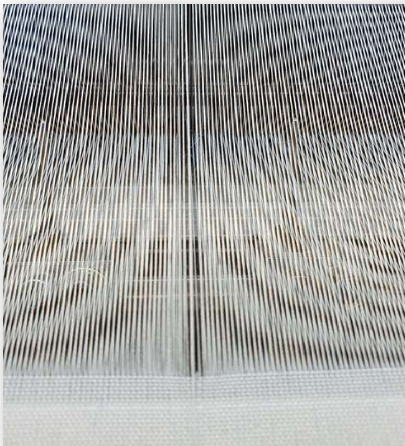
Wrong drawn-in defect in fabric formation zone
