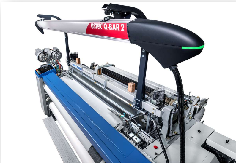
Uster Q-Bar 2 – The formation monitoring system
