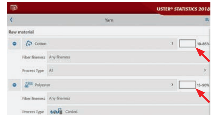
Fig. 1 Possible range for blend ratio selection in 1% steps. The indications and options change relative to the blending agents
