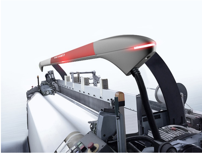
The next generation of on-loom monitoring and inspection: USTER® Q-BAR 2
