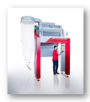
Uster Jossi Vision Shield – detection and elimination of natural and synthetic contamination
