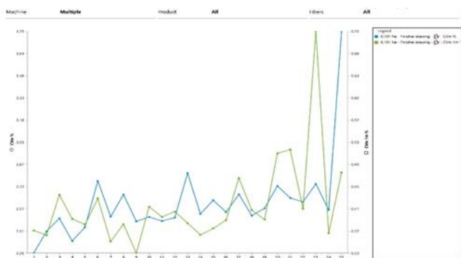
Fig. 2: USTER® QUALITY EXPERT analysis showing significant variations in sliver evenness (CVm) and CVm1m mid-term
