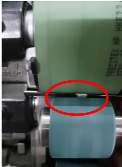
Fig. 1: The roving was misguiding, going above the pin bar spacer instead of underneath.
