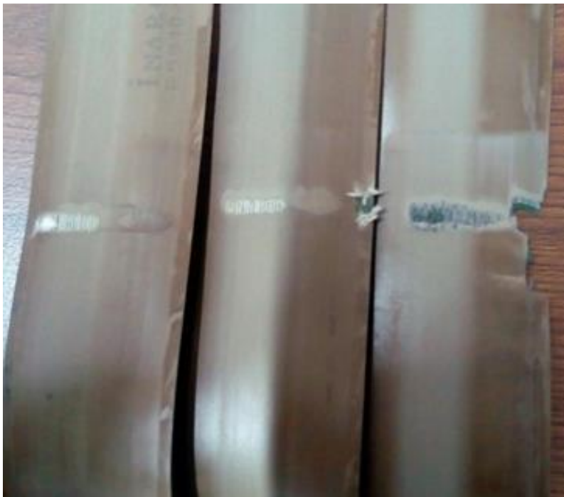
Fig. 3: Defective aprons which caused long mass variations, leading to an increase in CCp cut level.
