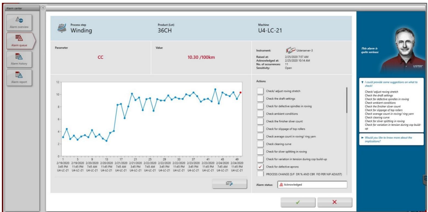
Fig. 1: USTER® QUALITY EXPERT screen showing the increase in CCp cuts to 8 -12 cuts/100 km.
