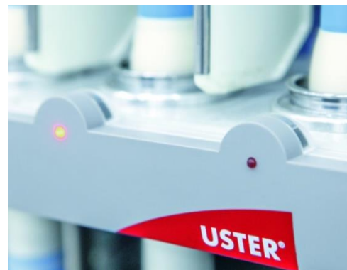
Fig. 2: LED of Uster Sentinel showing RSO 3D alarm.
