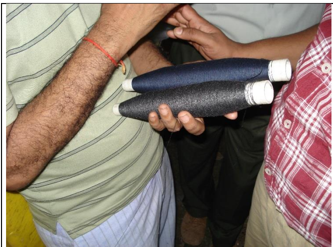
Fig. 20 Mix-up of 2 color shades using the same tube color
