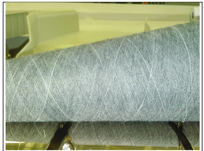
Fig. 21 Shade variation detected by the SV channel
