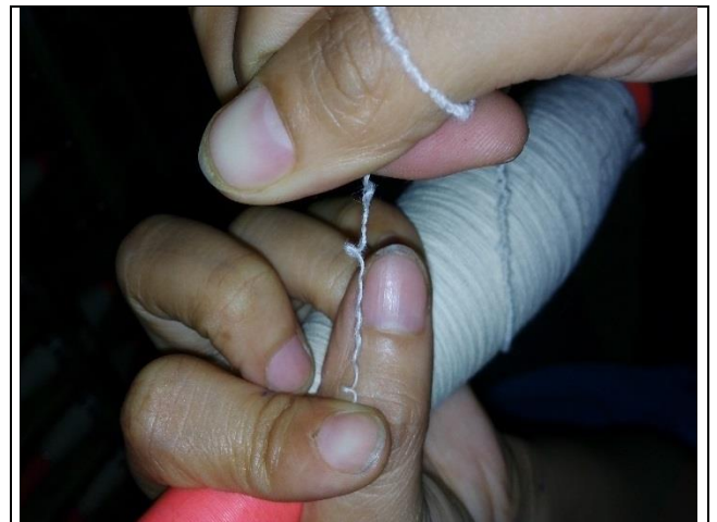
Fig. 27 Defective yarn with off-center core
