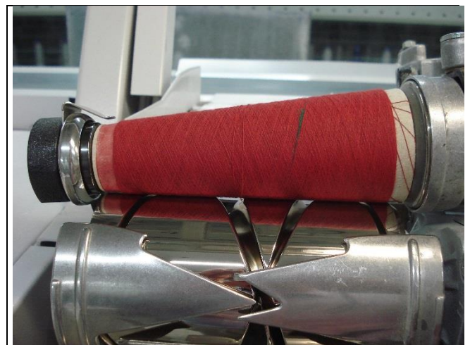
Fig. 13 Spun-in colored defect in colored yarn
