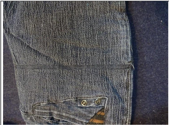
Fig. 22 Missing core resulting in fabric barré
