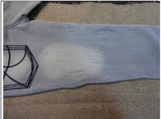
Fig. 23 Missing core leads to cloudy fabric appearance
