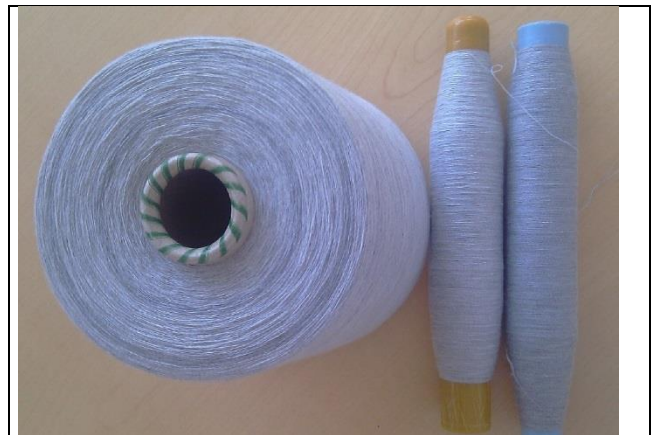
Fig. 17 Mix-up of different mélange shades
