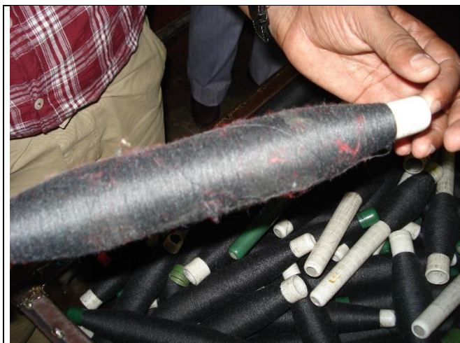
Fig. 12 Color contamination by fluff and fly
